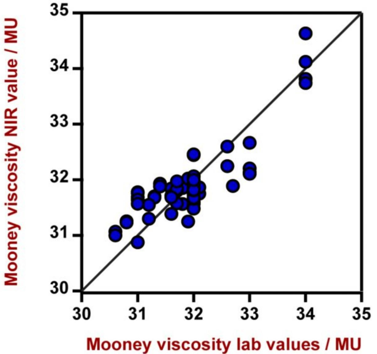
**Figure 3.** Correlation diagram and the respective figures of merit for the prediction of Mooney viscosity in BIIIR using a DS2500 Liquid Analyzer. The lab values were evaluated using a Mooney viscometer.
